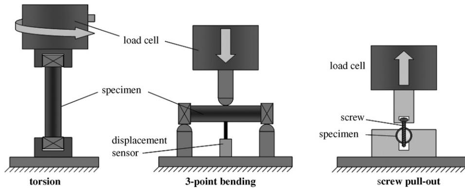
Fig. 2. Test configurations for structural property evaluation of bone surrogates in torsion, bending, and screw pull-out.
