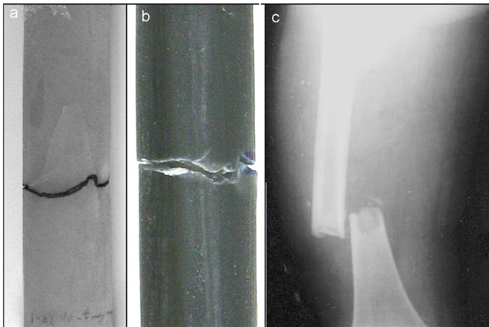
Fig. 5. (a) Bending failure of osteoporotic bone surrogate, (b) normal bone surrogate, and (c) in a femur shown on a clinical radiograph depicting transverse fractures typical for bending-induced injuries.
