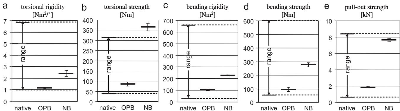
Fig. 3. Five structural properties for cadaveric femora (native, cumulative literature range), osteoporotic bone (OPB) surrogates, and normal bone (NB) surrogates: (a) torsional rigidity, (b) torsional strength, (c) bending rigidity, (d) bending strength, and (e) screw pull-out strength.
