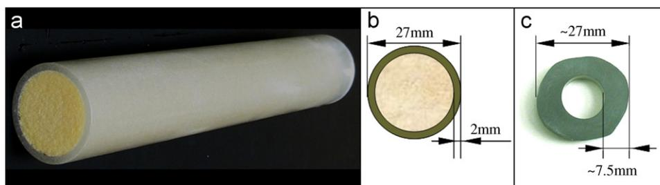
Fig. 1. (a) Osteoporotic bone (OPB) surrogate composed of a short e-glass fiber reinforced epoxy cortex and a polyurethane foam core, (b) cross-sectional geometry of OPB, and (c) normal bone surrogate in diaphyseal region.
