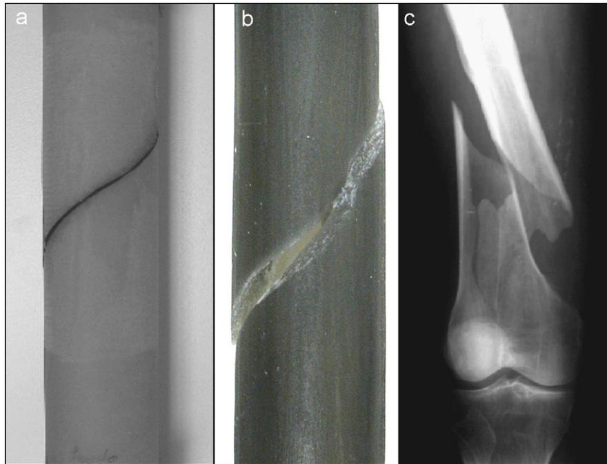
Fig. 4. (a) Torsion failure in the osteoporotic bone surrogate, (b) normal bone surrogate, and (c) in a femur shown on a clinical radiograph—depicting spiral fractures typical for torsional injuries.
